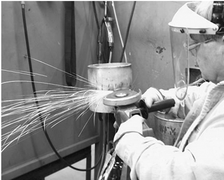
Fig. 3 Grinding of Weld Flaw
